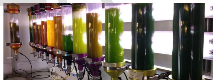
Figure 7 Cultivation of different algal species in bubble columns vertical tubular PBR at Plymouth Marine Laboratory [27].
